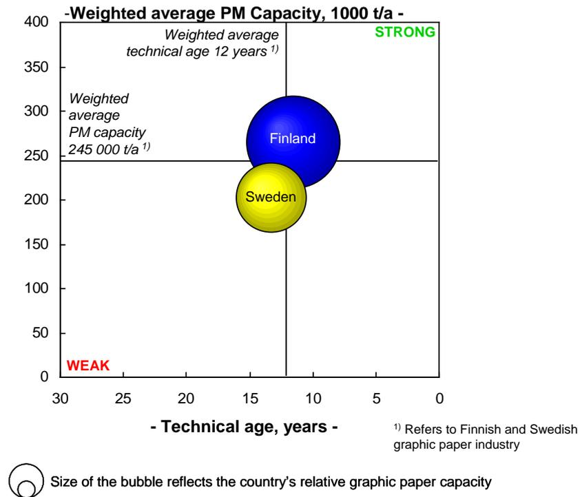
Figure 4. Technical comparison of the graphic paper machines operating in Sweden and Finland (Data provided by Jaakko Pöyry Consulting).
